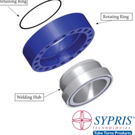
For Alignment of Flanged Piping
