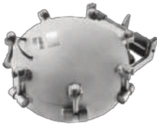
**T-Bolt Closures** are designed for nominal pressure applications. T-Bolt closures are available for horizontal and vertical applications in sizes 6" - 66" for pressures up to 300 psi.
