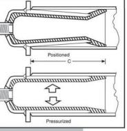
And when the test is finished, the SWEL-PLUG Pressure Tester can be removed with a minimum of effort because its grip to the pipe walls slackens automatically as internal pressure is relieved.
